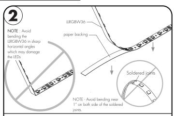
2.1 Remove the paper backing from the LLRGBW36 and firmly press down making sure there are no air bubbles that can cause surface irregularities. Do not remove the adhesive, removing the adhesive may cause arcing of the Line LED tape.
