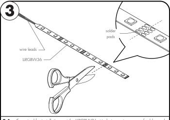
If required for installation, cut the LIRGBW36 strip between two rows of solder pads.
